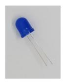
Take a look at one of your LEDs. The legs on it are two different sizes. The longer leg is the positive side (also known as *anode*) and the shorter leg is the negative side (also known as *cathode*).
