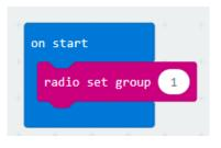
Move an on start block to the workspace. Under Radio, find the radio set group \_\_\_ block and connect it to the on start block.
