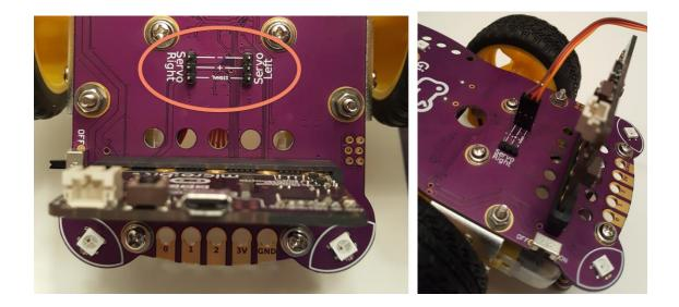
Ensure that the servos are connected properly. If the servos are not connected the correct way, they will not work. The brown wire (or black wire) needs to be towards the rear end of the GiggleBot.
